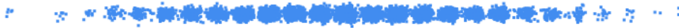
Fig. 1 The wave-like interference pattern (diffraction fringes) that is formed from the accumulation of all the 7019 electrons fired.
